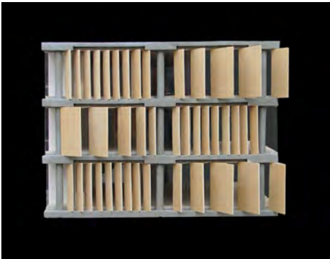
Working out the brise-soleils was crucial to the development of the project after the competition. We started out by working with simple right-angled panels
